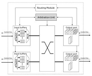
Figure 9. Typical virtual cut-throutgh router microarchitecture. The shaded areas are modified to implment the proposed Critical Bubble Scheme.
