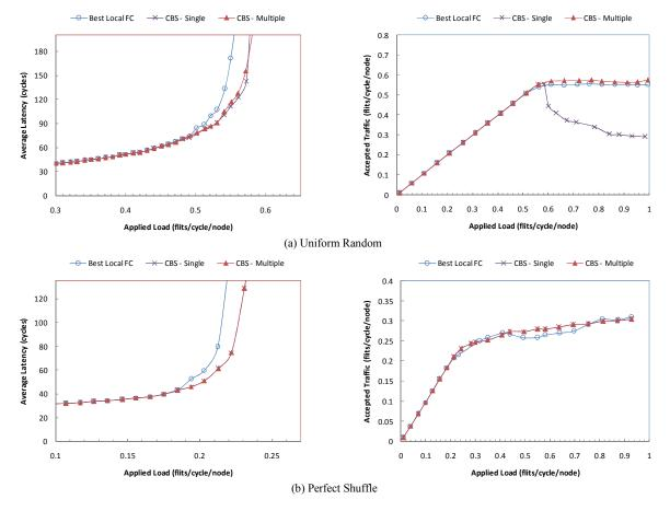
Figure 13. Effects of using mulitple critical bubbles for CBS under different traffic patterns.
