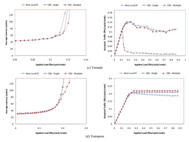
Figure 13. Effects of Using Mulitple Critical Bubbles under different traffic patterns.
